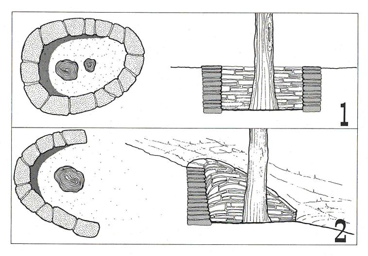
As in the case of an exterior planter, a tree well is a retaining wall around the base of a tree to hold back the earth when a change of grade is desired. If the earth were to cover the tree to the height of the embankment, the tree would die in a matter of months.
